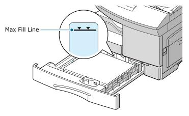
7 While squeezing the side guide as shown, move it toward the stack of paper until it lightly touches the side of the stack. Do not too tightly to press the guide the edge of the paper; the guide may bend the paper.
